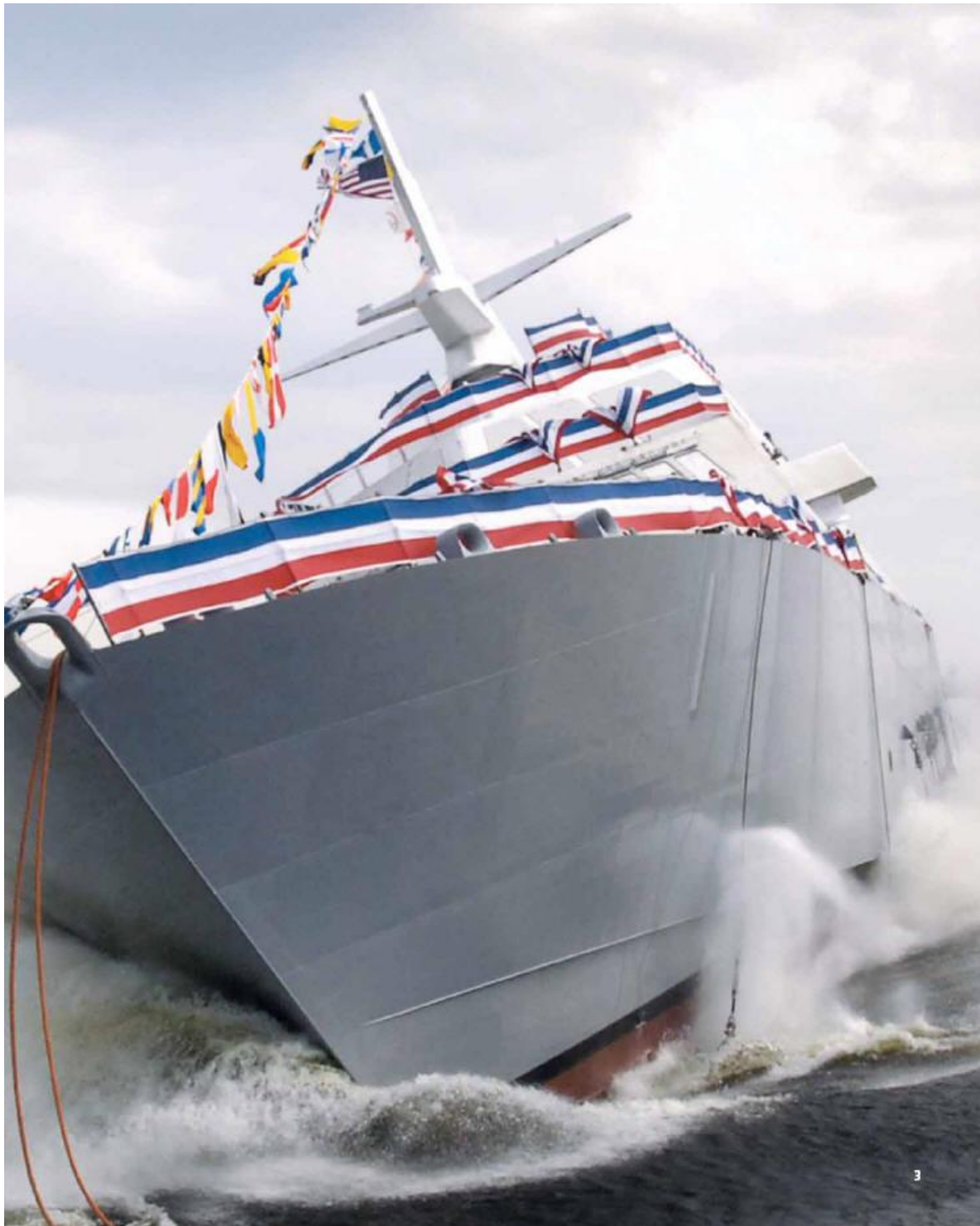
The Navy's new littoral combat ship PCU Freedom (LCS1) makes a spectacular side launch during her christening. Displacing 3,300 tons and with a capability of speeds of more than 40 knots, Freedom is designed with operational flexibility to execute focused missions such as mine warfare, anti-submarine warfare, surface warfare and humanitarian relief. Source: All Hands, December 2006
